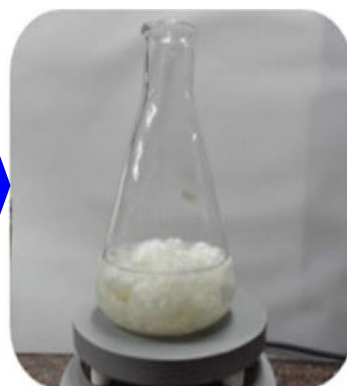
Degumming: removal of protein sericin
