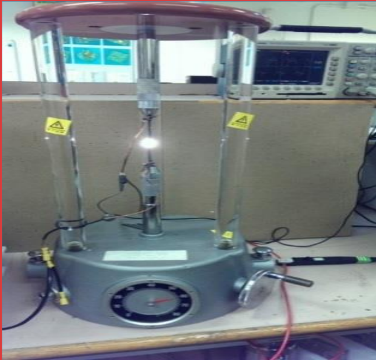
Carbon arc discharge in operation
