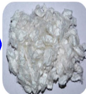
Degummed fibre of protein fibroin
