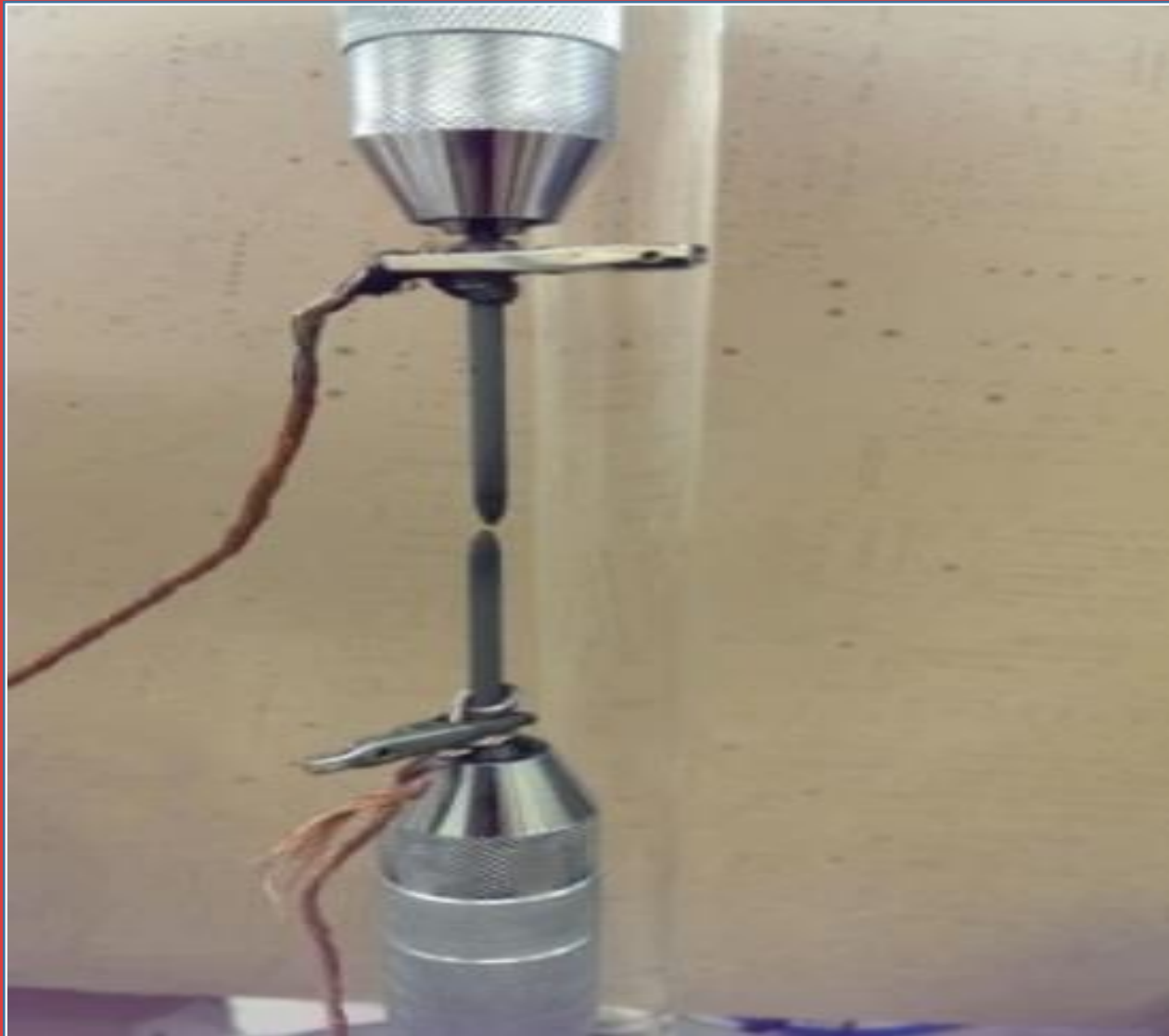
Setup of the carbon rod electrodes
