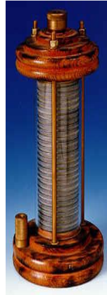
Voltaic Pile (Invented by Volta 1800)
